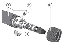
Replace the felt strip if the oil-laden return air that escapes is soiled. We recommend replacing the felt strip at least every three months.
