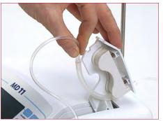
The compartment with the integrated tubing bracket opens smoothly and the tubing set can be fitted very easily all with one hand.
