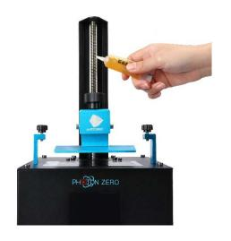
(1) If Z axis make noisy sound, please apply lubricant to Z lead screw.
