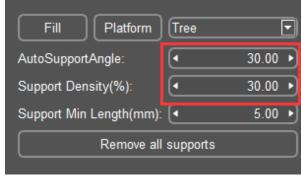
If we increasing the automatic support angle and support density (highlighted by red square), we can see from the picture below that more supports have been added to some of the weak points.
