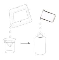
(4) Do not left the resin in the vat for over two days if not using it. Please filter and store the resin properly.
