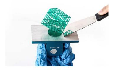
**[IMPORTANT]** In case of incomplete curing or failed prints, there might be some resin residues left in the vat. Then, please filter the resin by a funnel and store the resin in a sealed container. For the residues left in the vat or on the platform, please use paper towel or plastic scrapper to carefully get rid of that.
