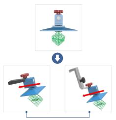
Tighten the platform securing knob
