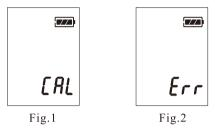
Press the on/off button ① to start or stop the calibration. When the calibration is initiated, "**[FIL**" Starts flashing on the display and starts counting down. (Fig.1)
