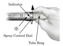
Turning the dial in the direction indicated by the arrow in the illustration will gradually reduce the amount of spray and then reach 0. For maximum spray, continue the turning the dial until the "W" matches up with the indicator. (See illustration.)
