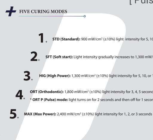
STD (Standard): 900 mW/cm<sup>2</sup> (±10%) light intensity for 5, 10, 15, or 20 seconds
