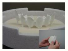
This method reduces the surface friction and allows the framework to <u>'slide</u>' on flat pins as it shrinks. Make sure to frequently polish the surface of the round zirconia plate by rubbing it with a grinding stone. This plate is from Katana, Noritake and works well to prevent "deformation" of your framework. (for DelCam and other open CAM software users)
