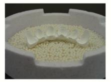
Ensure that the entire surface of the substructure is supported by the sintering beads. This avoids deformation. <u>Care should be taken to prevent</u> <u>sintering spheres becoming "jammed" in the connec-</u> <u>tor areas</u>. (for Sirona Cerec, MC-XL users)
