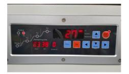
8. Select sintering schedule. 9. Confirm temperature and adjust if it is necessary
