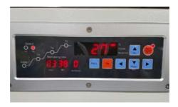
8. Select sintering schedule. 9. Confirm temperature and adjust if it is necessary
