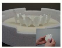
This method reduces the surface friction and allows the framework to 'slide' on flat pins as it shrinks. Make sure to frequently polish the surface of the round zirconia plate by rubbing it with a grinding stone. This plate is from Katana, Noritake and works well to prevent "deformation" of your framework. (for DelCam and other open CAM software users)
