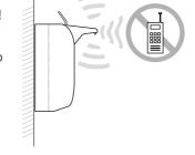
Electromagnetic interference sources and/or radiating electric fields may impair the function!
