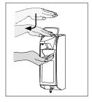
Approach the upper hand up to a distance of approx. 4 cm to the face shield - the dispenser actuates several times
