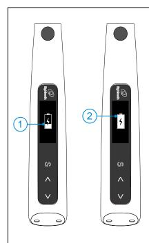
Charging indication appears on the screen, and flashes slowly  $(\bigcirc,1)$ , when battery is fully charged or in a state near full charge, the flash will stop and show like picture  $(\bigcirc,2)$ .
