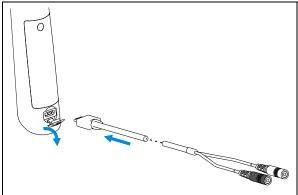
Insert lip hook into white slot, insert file clip into black slot.
