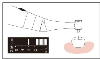
When using as a stand-alone motor, the torque bar will show on the screen (more information about torque bar, please see chapter 5.2 Screen display).
