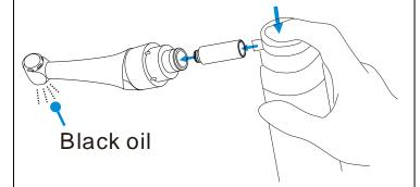
Before autoclaving, the contra angle must be lubricated.
