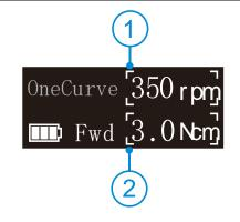
The parameters of "OneCurve" can also be changed make it different from default setting, and there will be 4 corners around the parameter  $(\bigcirc,1)(\bigcirc,2)$ .
