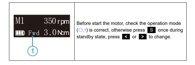
Operation Mode Fwd E-connect S has 4 operation modes: FWD, REV, REC and ATC (See chapter 5.3 Terms and definition to get the explanations of these modes).
