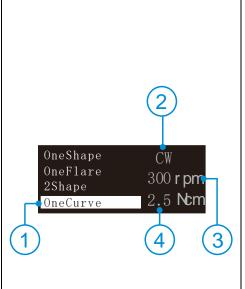
If you selecting "OneCurve"  $(\bigcirc,1)$ , the operation mode  $(\bigcirc,2)$ , speed  $(\bigcirc,3)$  and torque limit  $(\bigcirc,4)$  will change according to the file system default setting.
