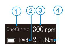
And the memory mode  $(\bigcirc,1)$  will change according, also operation mode  $(\bigcirc,2)$ , speed  $(\bigcirc,3)$  and torque limit  $(\bigcirc,4)$  will charge according to the file system default setting.
