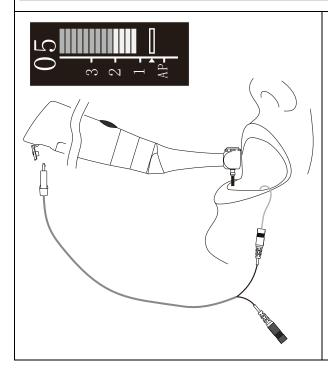
When using motor combine apex function, the measure wire must be connecting with motor by USB socket, and white slot connects with lip by lip hook, keep the black slot idle.
