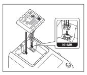
6 Refer to the figure below and place the battery into the battery chamber with care so as not to catch the cord.
