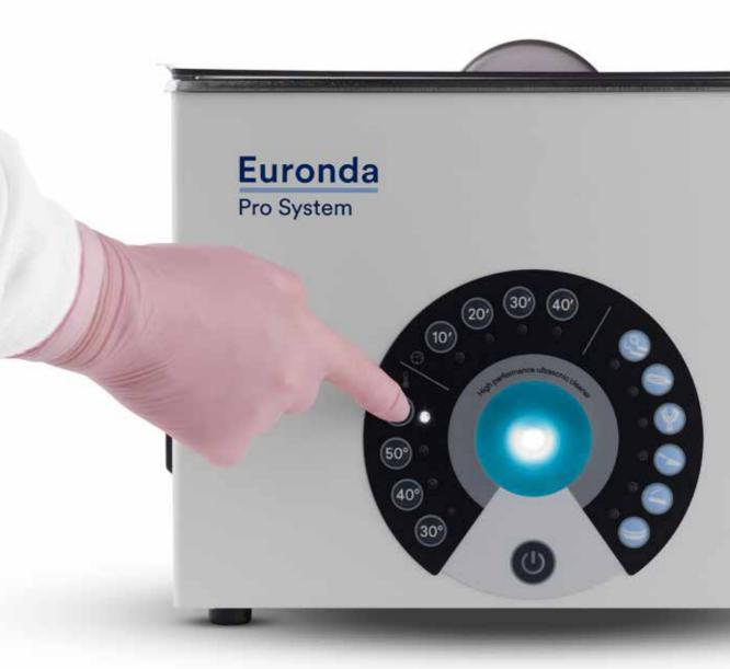
There are two operational modes, allowing users to choose one of the 6 preset cycles (instruments, burs, impression trays, cement removal, plaster removal, and prostheses) or run a free cycle at a temperature between 30°C and 60°C, with a duration between 10 and 40 minutes. There are 4 different operating stages in the 6 preset cycles: Degas, Boost, Normal and Sweep.
