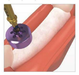
8. Insert Accurate Pin with the same size into the hole created after drilling.
