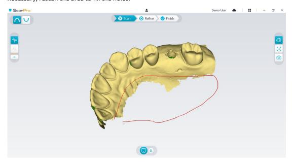
After scanning the upper jaw, you can continue scanning the lower jaw. On the ScanPro interface, select the Lower Jaw acquisition mode
