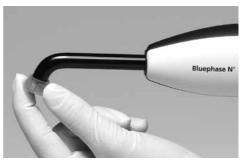
After that, mount anti-glare protection on the light probe.
