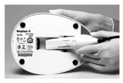
For this purpose, remove the battery from the handpiece. Then remove the power pack from the underside of the charging base. Do not pull on the power cord.
