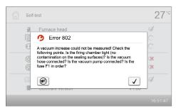
Press the [Continue] button to acknowledge the self-test.
