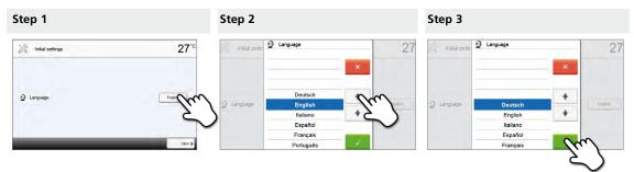
Select the desired language using the **[Arrow up/down]** buttons. Confirm the entry with the green button. By pressing the **[Continue]** button, you will reach the next entry screen.
