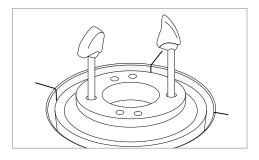
The crystallization tray must be placed in the centre of the object plate and within the circumferential groove in the object plate.
