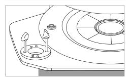
Remove the crystallization tray using the special tweezers and place it on the cooling tray.
