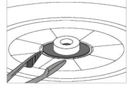
Always make sure that the correct temperature control ring UTH or MTH is used. The use of an incorrect temperature control ring results in damage to the object plate and other components in the firing chamber.
