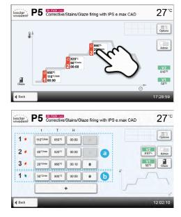
In the parameter view, the parameters can be changed. Up to three heating (a) and two cooling (b) stages are available.
