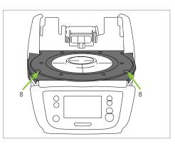
Place the cooling tray (7) on the frame plate (19). Make sure that the cooling tray is correctly positioned on the frame plate.
