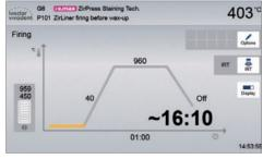
The IRT key (see Chapter 5.1.2) is used to switch to the view of the infrared camera during the closing and predrying process. The corresponding key is pressed again to return to the firing curve display.
