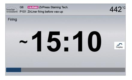
The factory settings of the furnace are such that the firing curve is automatically displayed upon the start of a program.
