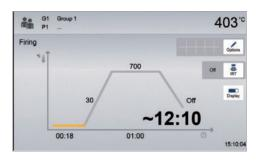
The IRT key (see Chapter 5.1.2) is used to switch to the view of the infrared camera during the closing and predrying process. The corresponding key is pressed again to return to the firing curve display.
