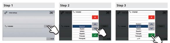
Select the desired language using the **[Arrow up / down]** buttons. Confirm the entry with the green button. The **[Next]** button is used to reach the next entry screen.
