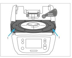
Place the cooling tray (2) on the frame plate (24). Make sure that the cooling tray is correctly positioned on the frame plate.
