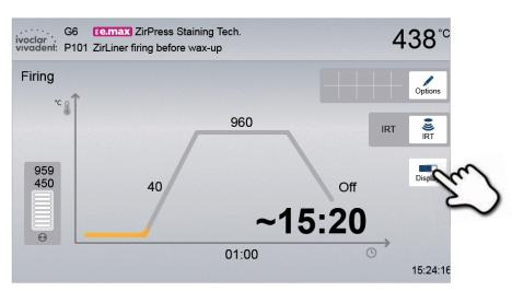
If the **[Display]** button is pressed while the firing curve is displayed, the remaining time will be shown. The remaining time indicator informs the user about the time that is left until the process is completed even from a distance. The remaining time is displayed in the center of the screen in large characters.
