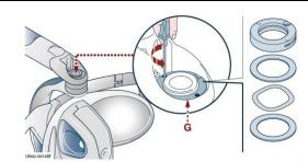
3 – Screw the safety screws F until the cut (A) into the brass nut is completely closed.
