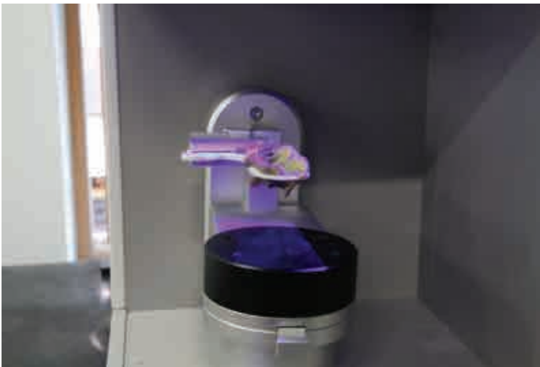
Put the impression on the impression jig and mount onto the scanner. Click "Auto Scan" 2 to proceed with scanning
