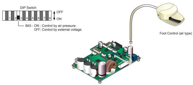
Insulate and bundle the wires which are not being used to avoid short-circuit.
