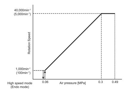
In the case of Multi Pad control, the air pressure of the motor start and maximum speed can be adjusted in the setting menu of Multi Pad.
