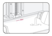
Shake the resin bottle for 1 minute. When pouring, make sure the resin does not exceed the mark on the resin vat.
