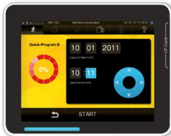
Time pre-selection for automatic autoclave start
