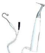
Fig: connect the lip hook to the white end of the measuring wire and keep the black socket idle if using the function of endo preparation accompany with apex locating.
