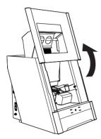
3 Orient the parts as shown in the figure, and then insert the adapter into the clamp.
