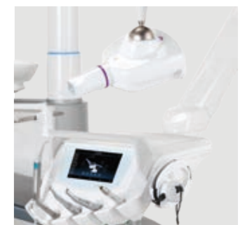
RXDC - HyperSphere technology Incorporated on the dental unit, the X-ray unit and handheld control unit require no additional installation points. Thanks to a combination of 30 cm collimation and a 0.4 mm focal spot, parallelism is excellent and images are pin sharp. Locked and unlocked by touch-sensitive pads, the tube head rotates freely around the spherical joint.
