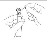
Use the nozzle needle (Mat. no. 0.410.0931) to free the water passage at the spray tubes.
