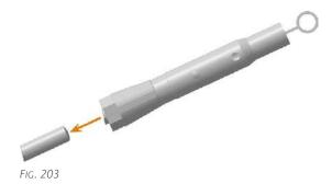
6. Clean and grease the collet chuck and reinstall it:
