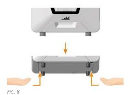
11. Lift the machine out of the padding.
