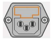
FIG. 190 COVER OF THE FUSE (MARKED ORANGE)
