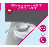
Temperature difference outside of the adjustable range. Repeat test firing. Contact dealer.
