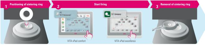
Place the sintering ring without sintering beads in the center of the sintering tray\*.
