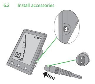
Plug the measuring wire into the socket of the device.
