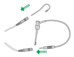
Insert the lip hook and file clip into the other end of the measuring wire.
