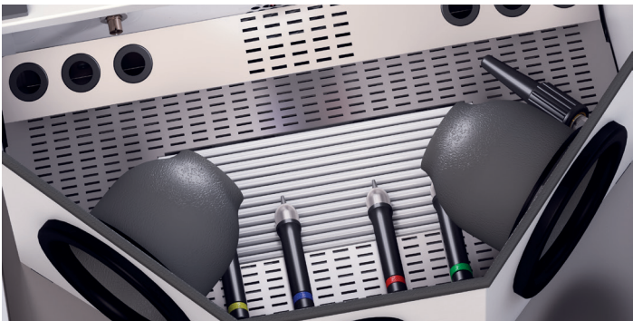
Ergonomically shaped handpieces and a separate air blasting nozzle
