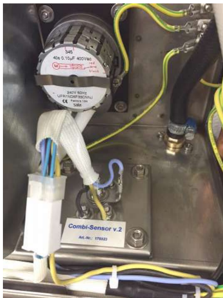
The combi-sensor v.2 (REF 170323) is located below the cleaning roller (slightly off to the right).
