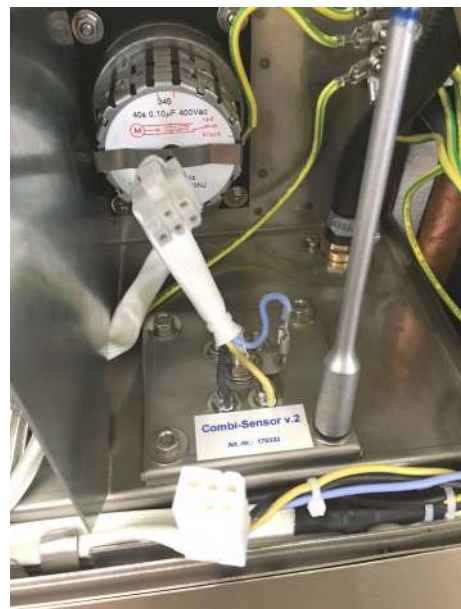
(4x M5) unscrew the nuts
