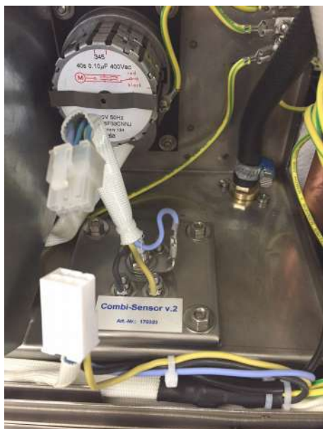
Pull off the sensor plug (6-pin)
