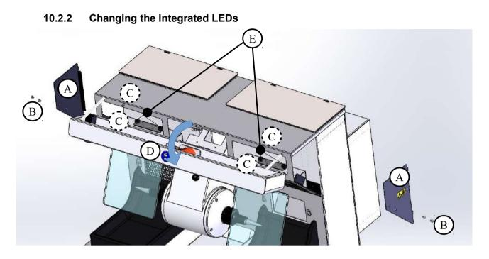
Disconnect the power plug before starting any maintenance work.
