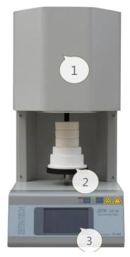
①: Sintering Furnace ②: the Bottom Tray ③: Touch Screen Control Panel
